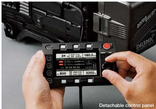
Detachable control panel
