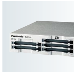
AJ-PCD35 "P2 drive" Memory Card Drive High-speed PCI Express interface.
